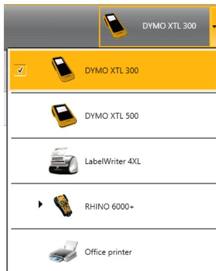
If you have more than one label printer installed on your computer, you need to select the appropriate label printer before printing.
